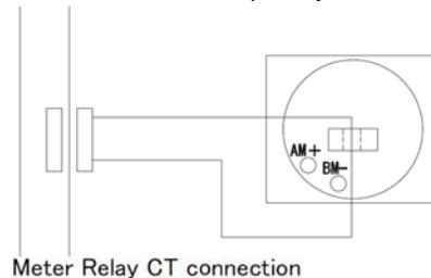
Since AM+ and BM- are non-contact, they can be used as relay terminals.
